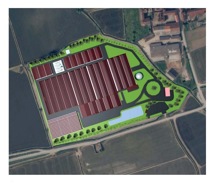
The plant uses a combination of an anaerobic (digestion) and aerobic (composting) processes for the treatment of source separated organic waste, food waste, green waste, sludge and municipal organic waste with recovery of electric energy and matter (compost).
