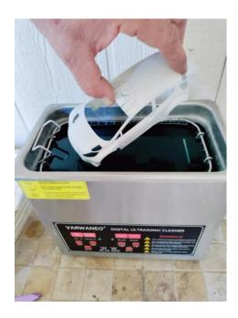
The model had about three coats of primer on it with another three thin coats of gloss white. At first nothing happened, but after twelve hours the paint bubbled in a few places, and I just let it keep soaking it and agitating it with the ultrasonics from time to time. Now, without any scrubbing other than the ultrasonic type, the body is as you see it here.
