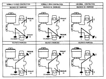
NOTE: PORT MARKINGS 1, 2 AND 3 CORRESPOND DIRECTLY TO A, B, AND C.
