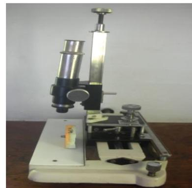
Cast Crown In Traveling Microscope For Evaluation
