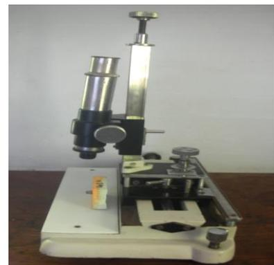
**Cast Crown In Traveling Microscope For Evaluation**
