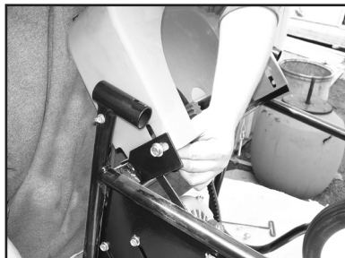
Step 9 • Paso 9 • Étape 9 Attach orange guard as shown with black bracket on the outside of the guard • Dije la guarda anaranjada como se muestra, con la ménsula negra por fuera de la guarda • Attach orange guard as shown with black bracket on the outside of the guard
