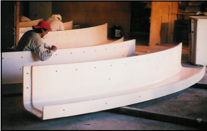
Curved Wall mounted trough Shows groove end of tongue and groove
