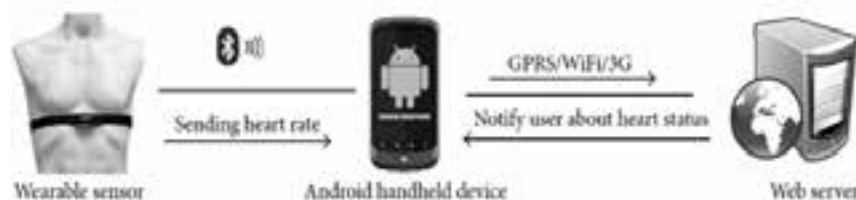
Figure 2 - A system architecture for remote monitoring
