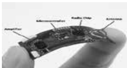
Figure 3 - illustration of Flexible wireless ECG sensor with a fully functional microcontroller[6]
