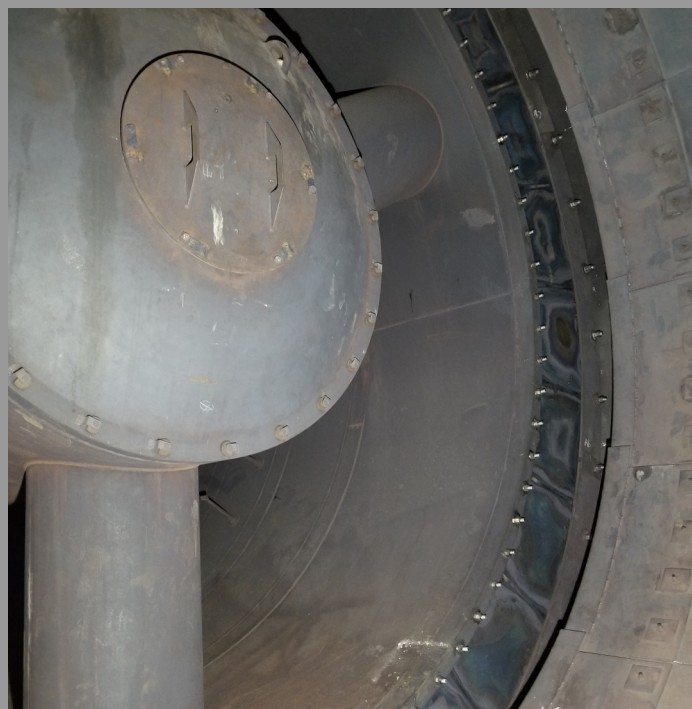
Complete Flex Seal, Gasket, and Hardware Replacement
