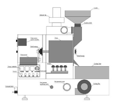
THE BC-2 IS A HEAVY DUTY ROASTER BUILT WITH A CARBON STEEL BODY WITH APPROVED POWDER COAT HIGH TEMPERATURE BODY IN BLACK, WHITE OR RED . THE HOUSINGS COME IN A CHOICE OF 4 COLORS AS LISTED BELOW.
