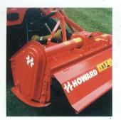
The trailing board's shape is specially designed for a perfect finish and an even flow of the soil
