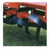
The four blade rotor works in hard conditions with a low power requierement.
