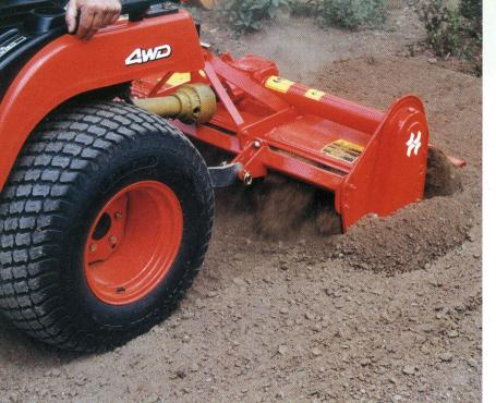
The machine is able to work up to 7 " providing a fine tilth and an even finish of the work
