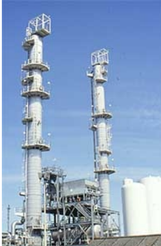
Alkylation Unit with Distillation Towers
