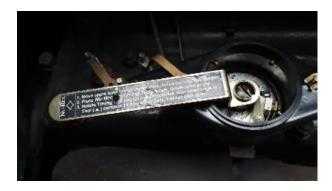
We drilled a hole in the handle of this tool that is lined up with pin #4 instead of the arrow. It is about half the width of the handle.
