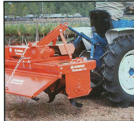
ROTA VATOR is designed for tractors with Category 0 or 1 - 3-point linkage.
