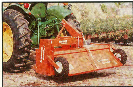
Twin depth-control wheels are standard on HJ 40", 50" and 60" models.
