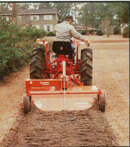
ROTA VATOR models are available in 32", 40", 50" and 60" tillage widths.
