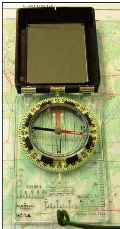
Figure 2 Set Compass to 00
