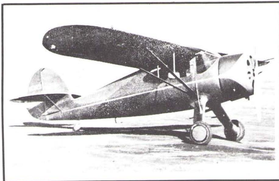
PHANTOM introduced all-metal fuselage to private aviation, was Warner-powered.
