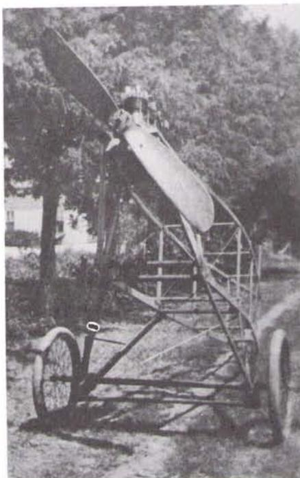
AIRFRAME view shows square fuselage, primitive engine. (33)
