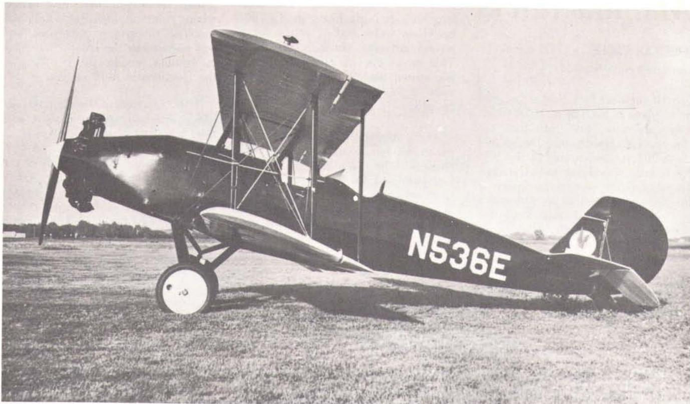
"ANTEATER" was nickname for A-129 with Kinner engine, which required lengthened nose to compensate for reduced weight. Aircraft pictured above belonged to Del Erhart, Lawrence, Kansas. It was destroyed by fire in 1967.
