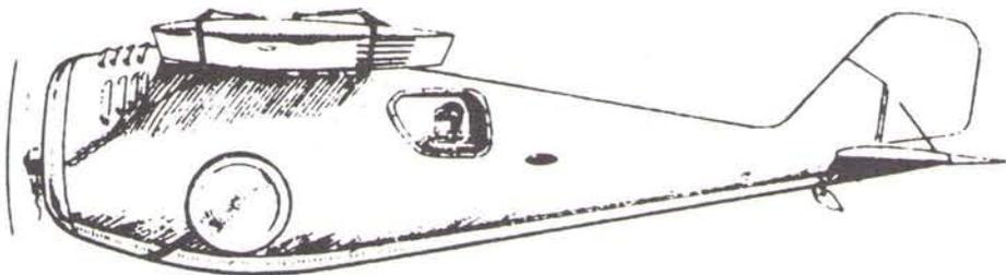
DAYTON-WRIGHT RACER was Bauman design, featured retractable gear and changeable-camber wings. (56)
