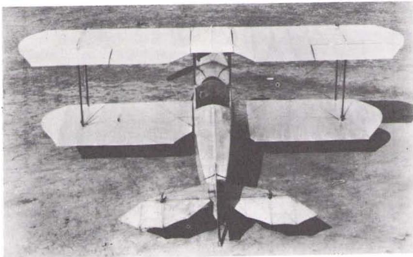
REAR VIEW shows scalloped elevator edges, "clean" instrument panel, with only ignition switch and oil pressure gauge. Original rudder fabric still checks out. (37)
