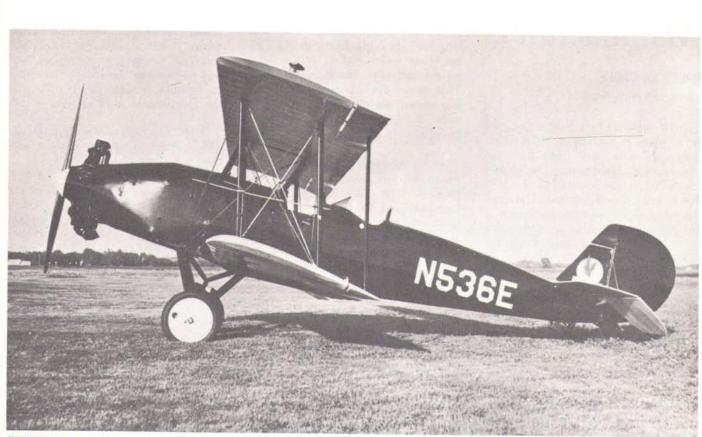
"ANTEATER" was nickname for A-129 with Kinner engine, which required lengthened nose to compensate for reduced weight. Aircraft pictured above belonged to Del Erhart, Lawrence, Kansas. It was destroyed by fire in 1967.
