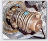
windings of the magneto. Follow the instructions in the *Ford Service Manual* to remove the Bendix and starter.
