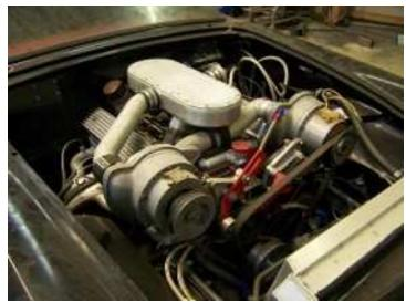
Yes – twin superchargers blowing into Hilborn fuel injection
