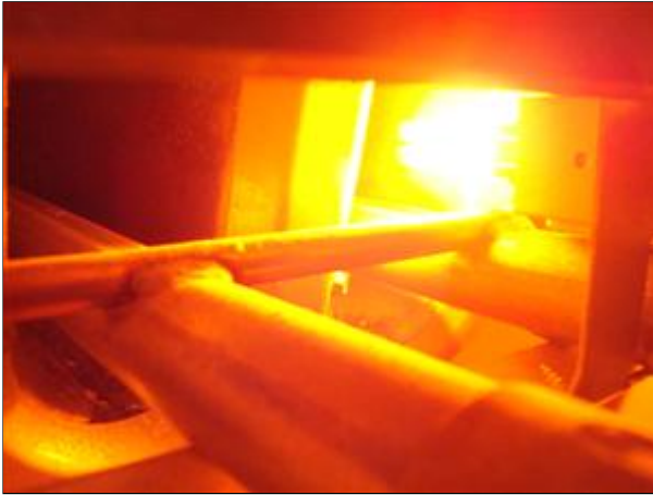
11.0 Picture 1 View of glow ignitor.
