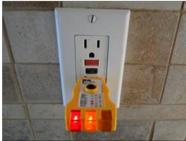
5.8 Picture 1 Hot Neutral reverse east wall.
