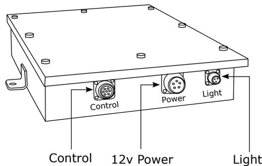
Control plug - the 7-pin plug is the receptacle on the actuator box that is connected to either the pendant or the optional extra wire plug.
