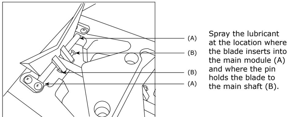
Spray the lubricant at the location where the blade inserts into the main module (A) and where the pin holds the blade to the main shaft (B).
