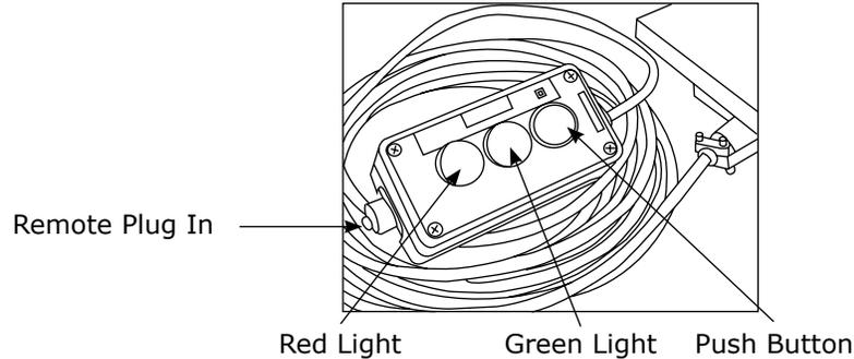
To lower the blades, depress the black button on the activation pendant again. The green light is now lit indicating it is safe for vehicles to pass over the system without harm to their tires. As long as the system is connected, the appropriate light will remain lit alerting the operator of the true status of the RoadBlade system.
