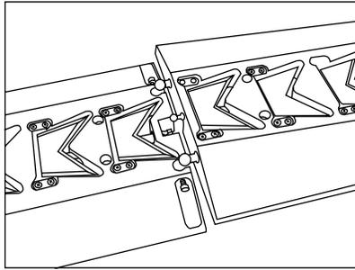
Once satisfied with the adjustments, lower the blades to allow the next module to connect with the previous module. Repeat this process until all of the modules for the RoadBlade system are attached. Lock the ball joints into the sockets using the 3/16" (4.762 mm) Allen wrench if the RoadBlade system is to be placed on the surface without anchoring. They are used to keep the system in a uniform manner.
