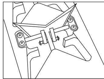
With the T-handle Hex Key unscrew the 4 mounting screws that hold the retaining plate against the blade's rotating arm. Insert a replacement blade. Replace the retaining plate and screw the 4 mounting screws back in.
