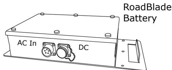
Battery - The two 5-pin plugs located on the battery are wired parallel to allow ease of use. Screw on the DC power cable onto the left receptacle to provide power to the RoadBlade system. The receptacle with the screw on cap is used to charge the battery. Before screwing on the AC cable to the receptacle place the cap on the other receptacle to prevent accidental shock.
