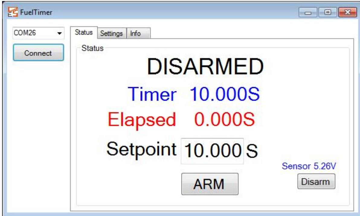
**COM PORT:** Com Port the timer is connected to. See device manager if unsure, *hint:* try the last one in the list as it will remember the last port it connected to.
