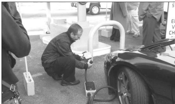
*Step two: Connect adapter to Tesla charging plug*
