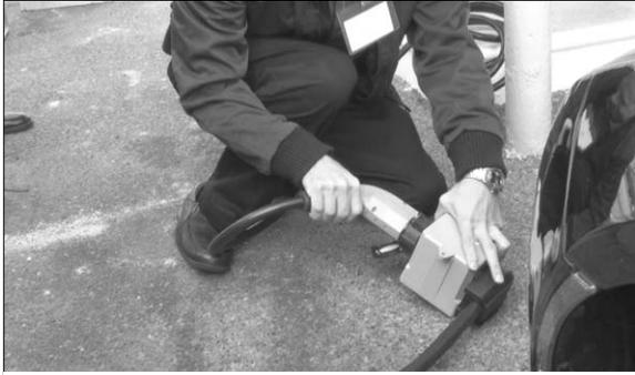
Step four: Plug J 1772 charging station plug into the adapter
