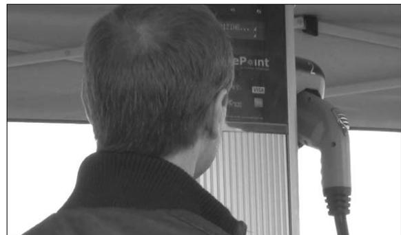
*Step three: Go to charging station and swipe a special card that will allow you to take the J 1772 charging plug out of its holder*
