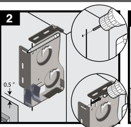
Mark bottom of slotted top hole on top of bracket. Drill 3/32" pilot hole on mark. If necessary, use wall anchor (not included). Secure brackets with one screw using a 1/4" driver.
