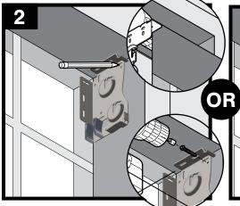
SIDE MOUNT: Mark bottom of slotted hole on side of bracket. Drill 3/32"pilot hole on mark. If necessary, use wall anchor (not included). Secure brackets with one screw using a 1/4" driver.
