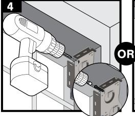
SIDE MOUNT: Drill second 3/32" pilot hole. If necessary, use wall anchor (not included). Secure brackets with second screw using a 1/4" driver.
