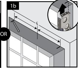
Find and mark center of opening. Mark top of window jamb on each side of window 1/2 the bracket-to-bracket dimension for the shade. Align outside edge of bracket with mark.
