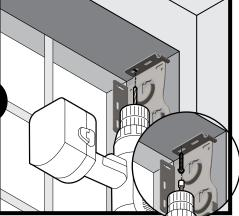
TOP MOUNT: Drill second 3/32"pilot hole. If necessary, use wall anchor (not included). Secure brackets with second screw using a 1/4" driver.
