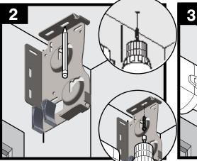
Mark center of slotted front hole on top of bracket. Drill 3/32" pilot hole on mark. If necessary, use wall anchor (not included). Secure brackets with one screw using a 1/4" driver.
