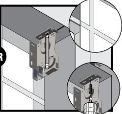
TOP MOUNT: Mark center of slotted front hole on top of bracket. Drill 3/32" pilot hole on mark. If necessary, use wall anchor (not included). Secure brackets with one screw using a 1/4" driver.
