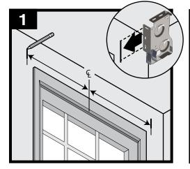
Mark center of opening. Make marks on wall on each side of window 1/2 the bracket-tobracket dimension for the shade. Align outside edge of bracket with mark.
