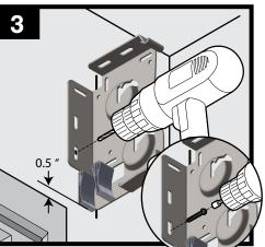
Dry fit top shade and check vertical side gaps and if shade is level (see Step 3 on page 2). Drill second 3/32"pilot hole. If necessary, use wall anchor (not included). Secure brackets with screw using a 1/4"driver.
