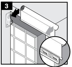
Dry fit top shade and check vertical side gaps and if shade is level. Adjust brackets if necessary by loosening screw and moving bracket down in slot. Once level, remove shade and tighten screw.
