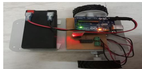
Fig.12. Prototype wheelchair Model controlled by control Commands from LabVIEW
