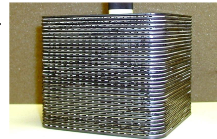
Electrochemical Stack (4" x 4" x 4")
