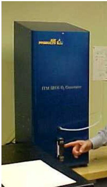
Solid Electrolyte Oxygen Separator 5 Liters/Minute (LPM) Breadboard
