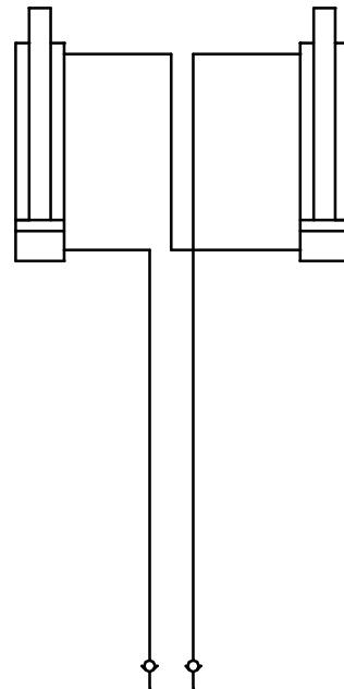
**Sistema hidráulico para control eléctrico de profundidad****3,0 m + 3,5 m**
