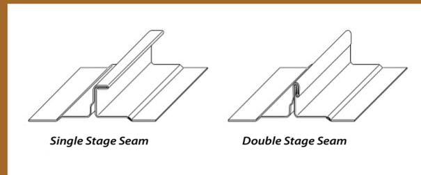
Standing seam panels can be seamed as a single stage seam or as a double stage seam, using a hand crimper or power seamer.
