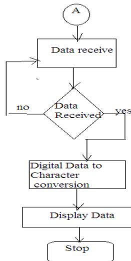
Fig.4: Flow Chart of Receiver side
