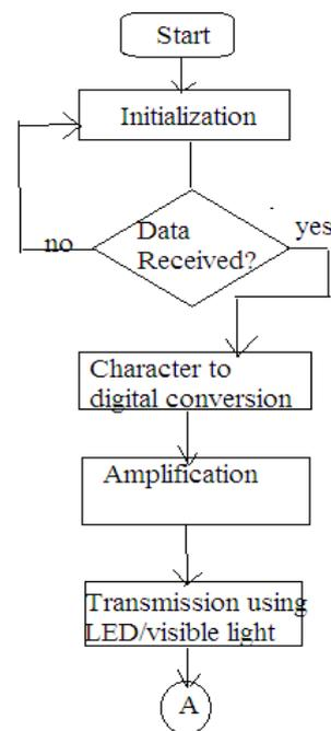
Fig.3: Flow Chart of Transmitter side
