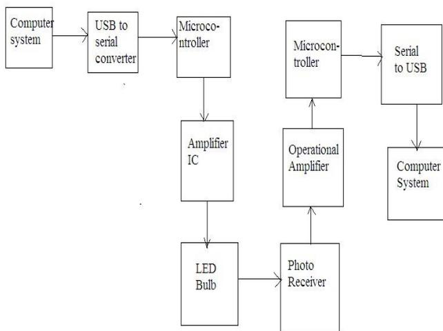
Fig.5:Data Flow Diagram Of Li-Fi Data Transmission
