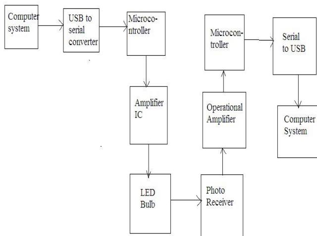
Fig.5: Data Flow Diagram Of Li-Fi Data Transmission
