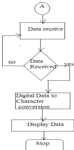
Fig.4: Flow Chart of Receiver side
