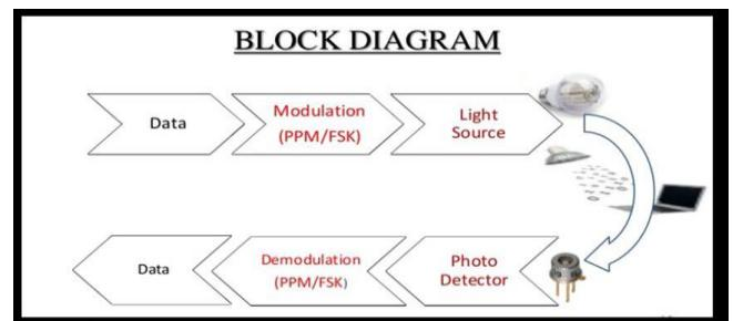
Fig.1: Block Diagram of Li-Fi Technology
