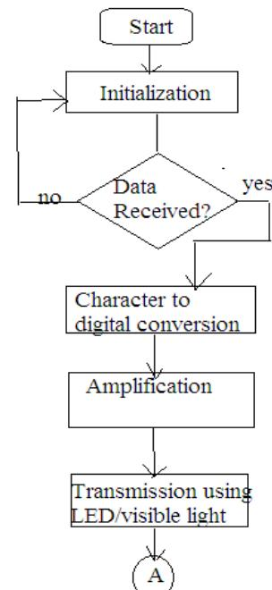
Fig.3: Flow Chart of Transmitter side
