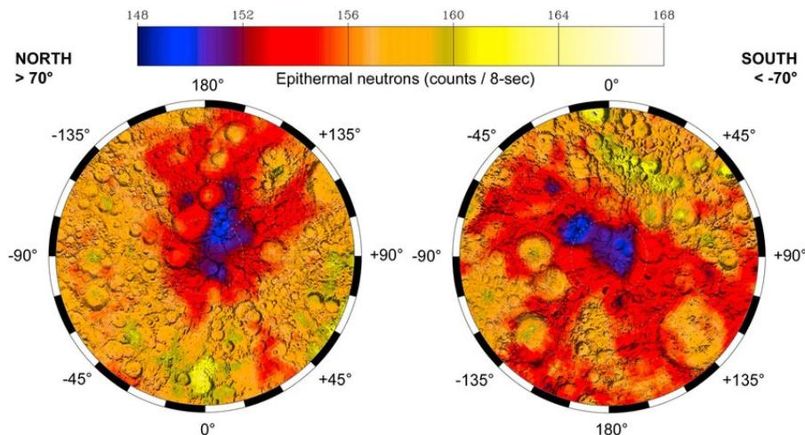
Figure 1 – Maps of [epithermal](#) neutrons for the north (left) and south (right) poles measured by the Lunar Prospector Neutron Spectrometer. From [Review Article \(10.1002/2016JE005167\) Figure 4](#). Courtesy of Reviews in Mineralogy and Geochemistry.
