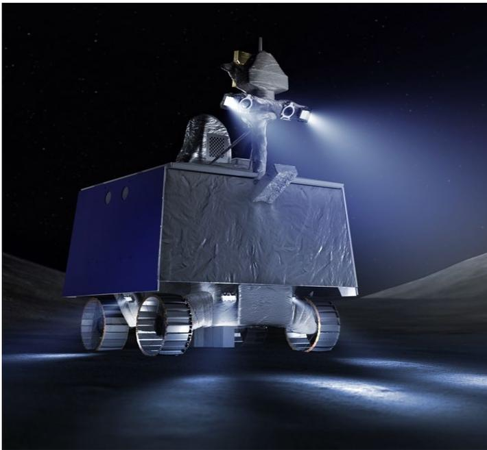
Figure 2 – The VIPER rover with cameras and lights in the front, back and near each wheel to allow for safe roving under all lighting conditions.
