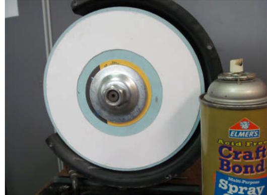
Adhere the paper disc to the outboard side of the wheel using photo mount spray.
