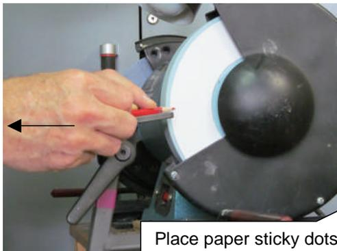
Place paper sticky dots between the edge of the cup washer and the outboard side of the wheel
