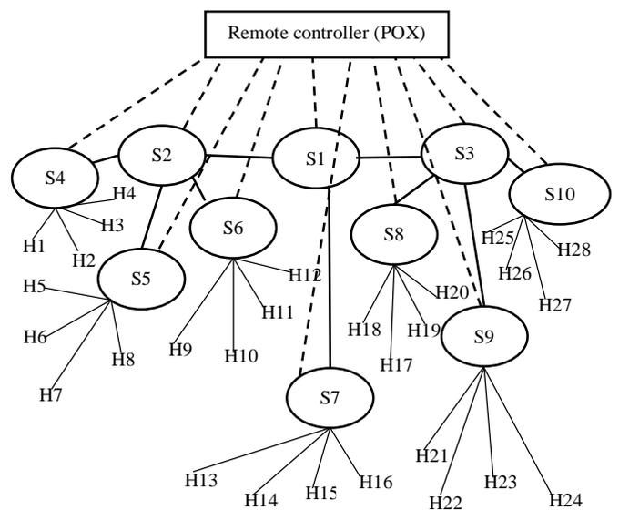
Fig. 4. Proposed OpenFlow based network model
