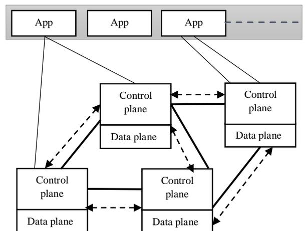
Fig. 1. Simplified Architecture of Traditional Network
