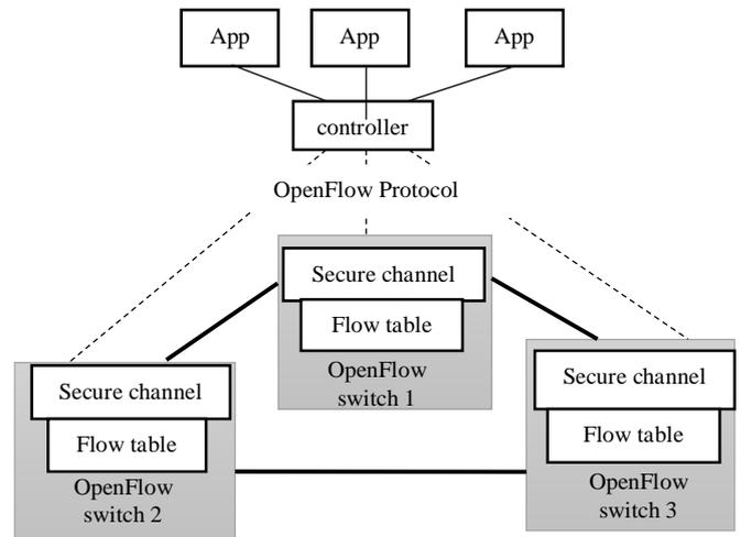
Fig. 3. OpenFlow based network architecture
