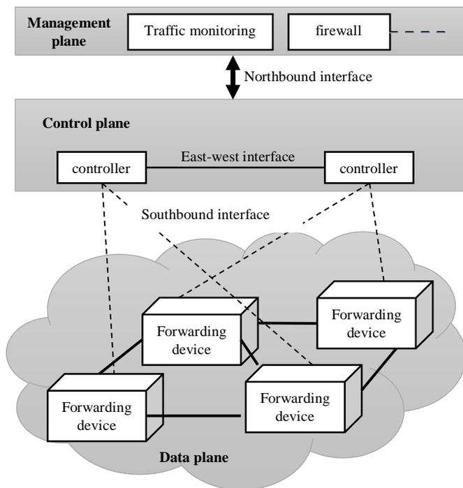
Fig. 2. Simplified Architecture of SDN
