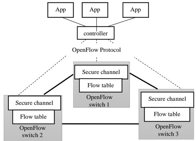
Fig. 3. OpenFlow based network architecture
