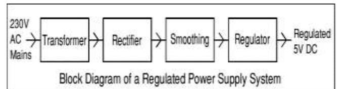
Fig. 3. Block diagram of power supply unit
