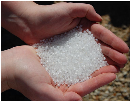
Thermoplastic resin pellets or “nurdles”. (Photo credit: left, public domain; right, International Pellet Watch)
