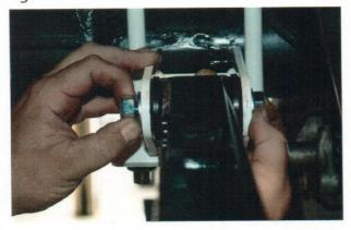
**10.** Assemble shackle to frame mount using another 1/2" x13x 4.75" bolt with washer, going through the frame mount and shackle.
