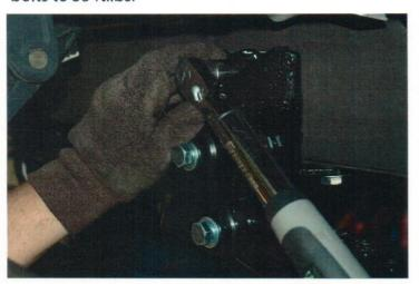
**24.** Install traction bars in place using provided hardware.
