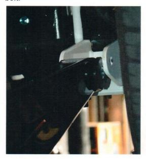
**9.** Install bolt with washer and toplock through the traction bar mount on the backside. Do not tighten.
