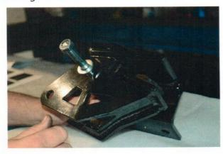
**11.** Place washer and toplock nut on the backside. **12.** Assemble shackle to traction bar using a 1/2"x13x4.75" long bolt.
