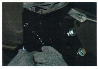
**19.** With the frame mount snugged down, mark the 3 side holes and the front bottom hole using a 1/2" center punch.
