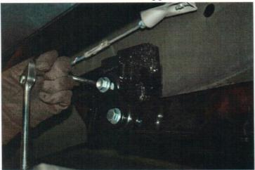
**23.** Reinstall shackle to frame mount. Torque all bolts to 55 ft.lbs.
