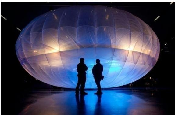
The inflatable part of the balloon is called a balloon swirl(envelope) .Loon’s balloon envelopes are made up from sheets of polyethylene plastic and they measure 15m wide and 12m tall when fully inflated. At the time of taken balloon out of the service gas is released from the envelope In the unlikely event that a balloon drops to quickly and parachute attached to the the of envelope is deployed.
