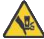
Crush Hazard SAX390 SAX391
