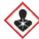
Severe Health Hazard SDN444 SDN445
