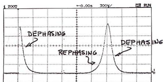
Figure 6 – Oscilloscope Trace Showing Spin Echoes
