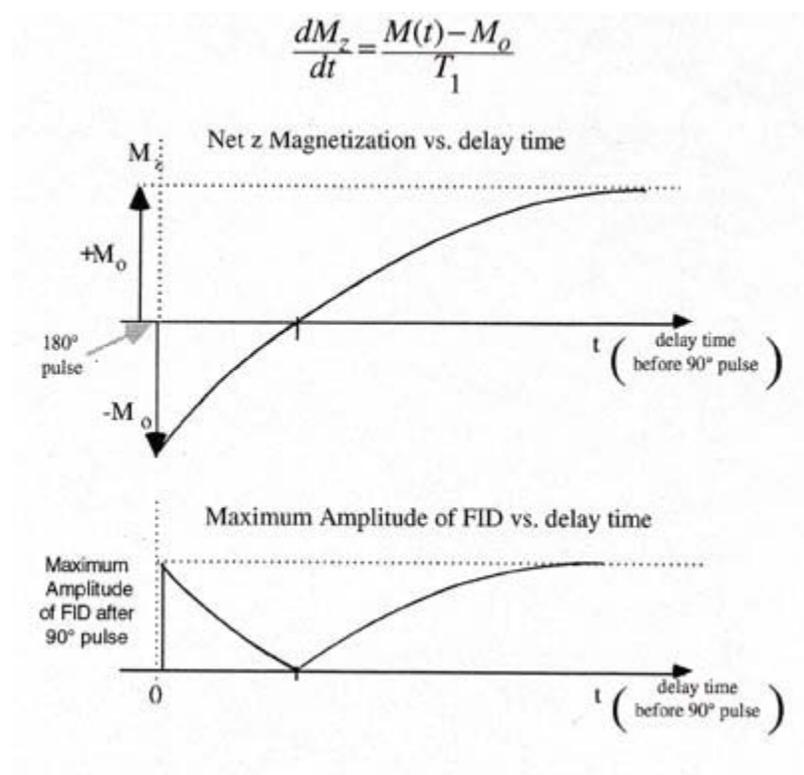
**Figure 5** – Upper Diagram: Net z magnetization vs. delay time
