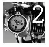
Firmly press your new OTB cover in place and screw in the top bolt. Hand tighten it to hold it in place. Then, do the same for the bottom bolt.
