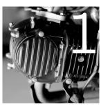
After removing the two bolts, remove the OEM timing gear cover.
