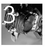
Your new OTB cover is designed to fit tight. Using your 8mm wrench, screw in the top bolt one full revolution and then screw in the bottom bolt one full revolution. Repeat this process top and bottom until both bolts are tight. This assures your new cover goes in straight and will not leak. The new cover should be tight against the motor housing when you are done.
