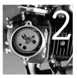
Firmly press your new OTB cover in place and screw in the top bolt. Hand tighten it to hold it in place. Then, do the same for the bottom bolt.
