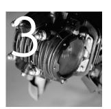
Your new OTB cover is designed to fit tight. Using your 8mm wrench, screw in the top bolt one full revolution and then screw in the bottom bolt one full revolution. Repeat this process top and bottom until both bolts are tight. This assures your new cover goes in straight and will not leak. The new cover should be tight against the motor housing when you are done.
