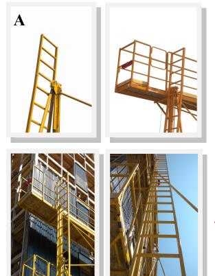
(A). <u>3' Ladder Extension</u>: is to raise the top of the ladder with the top handrail on the Main Platform.
