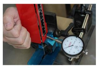
The blade guard on a bandsaw is not only an important safety factor but serves as a key component to supporting the blade as it is stressed during cutting operations.
