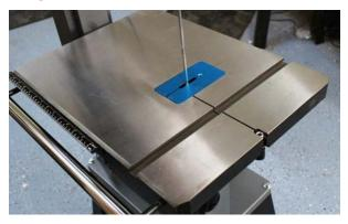
The 344 square-inch cast iron table provides plenty of working real estate. The system for attaching the table also includes a unique undocumented leveling mechanism that allows the table flatness to be perfected at installation time if any variance was present at the time of manufacturing. The table on the saw that we received was within .002" across its width so we did not find it necessary to make adjustments.
