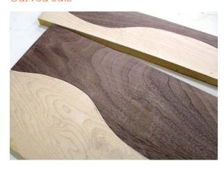
Band saws are commonly called upon to make gentle curved cuts in a work piece. While the radius of curve that can be cut is predominately determined by the width of blade, the cut quality is also influenced by the quality of guides, rigidity of the frame, and the structural integrity of the blade guard.
