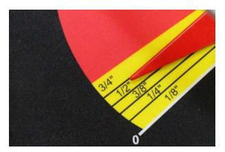
Differing from those found on most other bandsaws, the tension scale on the 1412 is easily readable, solidly constructed, and in our tests it actually proved to be a reliable guide for tensioning blades. Many woodworkers have differing philosophies on how a bandsaw blade should be tensioned, but regardless of the approach used, the tension gauge on the 1412 can serve as a good starting point or means of validation, eliminating much of the time and guesswork from the blade setup process.
