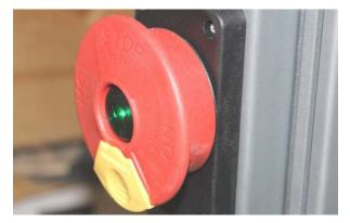
The switch design on the 14112 caught our attention. It is not the "run of the mill" two button unit that is found on most bandsaws, but rather an innovative single button design with a convenient light that indicates when the unit is powered. The operation requires a simple but conscious pulling action to ensure safe starting, and provides a large contact surface for easy "elbow operation" to halt the saw in a panic situation.
