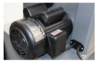
Rated at 1-3/4 horsepower, the motor delivers considerable resaw power for a bandsaw that can be used with normal household 110V 20 amp service. We performed our tests using a 20 amp circuit and measured actual amperage draw at 4.5 amps when running idle, and approximately 16 amps when we pushed it through a heavy resaw cut. The motor can also be optionally wired for use on a 220V service.
