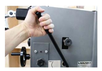
Once the tension is appropriately set for a given blade, the tension can be released and reset using the quick-release blade tension lever. While this has become a popular feature on many bandsaws in recent years, there are a couple noteworthy advantages to the implementation on the 1412. First, the handle is much longer than the handle found on many other bandsaws in this class, delivering
