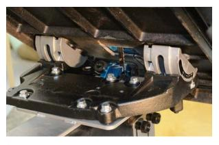
The table angle is adjusted by releasing two mechanisms that hold the table solidly against each trunnion. Each mechanism is released independently, and when loosened, the table is easily pivoted smoothly into position and re-locked. We checked the table's angle gauge with a digital angle gauge and it proved to be accurate to +/-.2 degrees.
