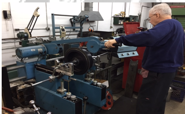
Flywheel in the balancing machine with Ray bringing it up to 700 RPM
