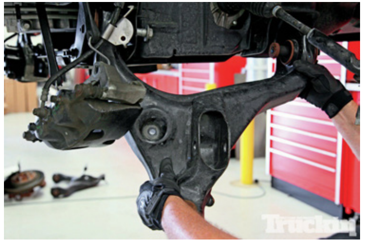
8. The F-150's lower control arms were next on the removal list.
