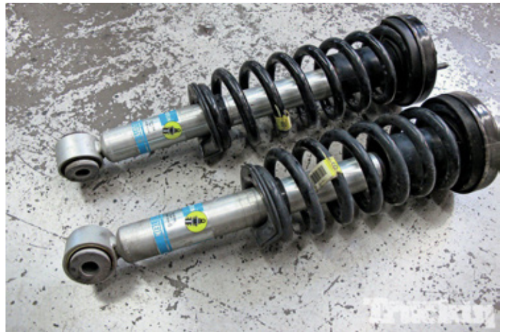
15. Even though we could have left the additional two inches in place on the Bilstein struts, the decision was made to drop the spring setting to stock to assess the truck's lifted height unassisted.
