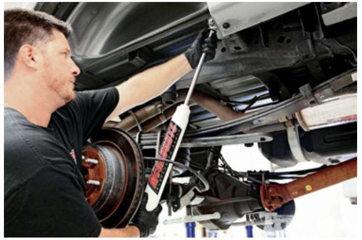
26. Extended-length gas charged shocks were bolted between the shock mounts.
