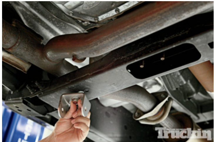
21. To prevent the taller crossmembers from moving, compression struts were employed. A threaded insert was slipped inside the transmission crossmember to accommodate the rear mounts.
