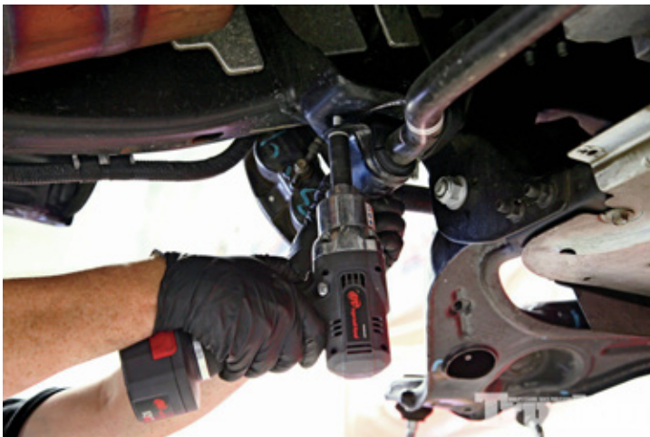
7. Using an Ingersoll Rand electric impact again, the front sway bar was disconnected and dropped from the frame.
