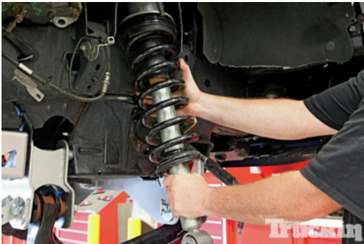
18. Even with the added height of the new upper mount, the strut assemblies could be set right into place.
