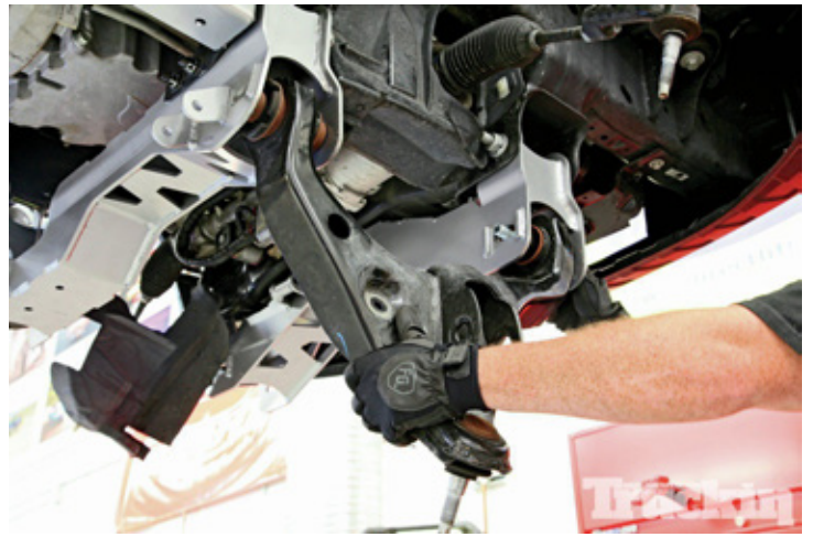
14. Getting the truck aligned was going to be easy since the kit was designed to offset the lower control arms with eccentric cams.
