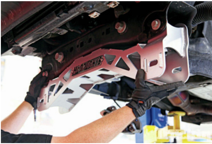
11. Original hardware held the new front crossmember into the frame mounts where the control arms used to reside.
