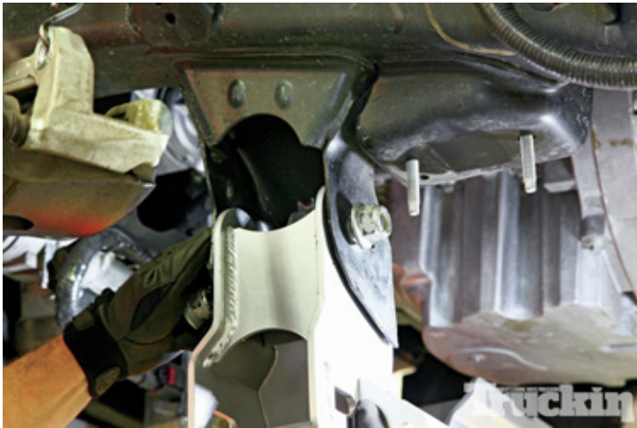
12. The rear crossmember slipped right into the previously chopped mount with the stock bolts.
