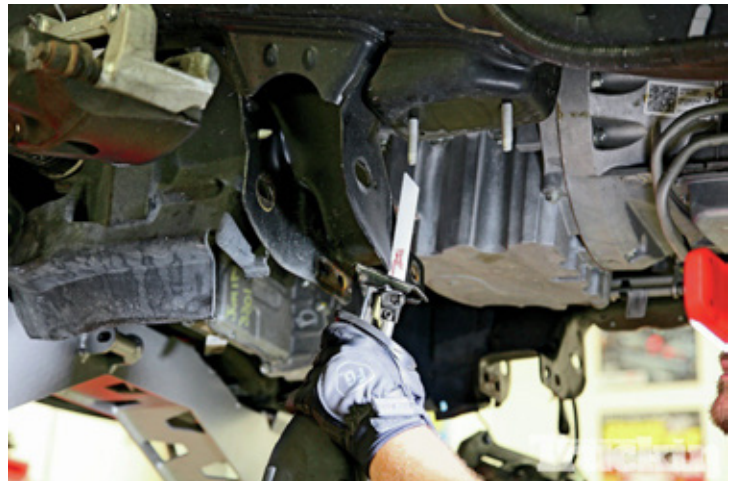
10. The "foot" on this frame mount was in the way of the McGaughys crossmember's new placement. Following the instructions included with our lift kit, it was cut off with a reciprocating saw.
