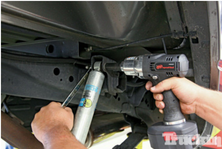
24. Installing the rear suspension lift was a quick affair. First the shocks were removed.
