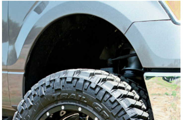
26. Extended-length gas charged shocks were bolted between the shock mounts.
