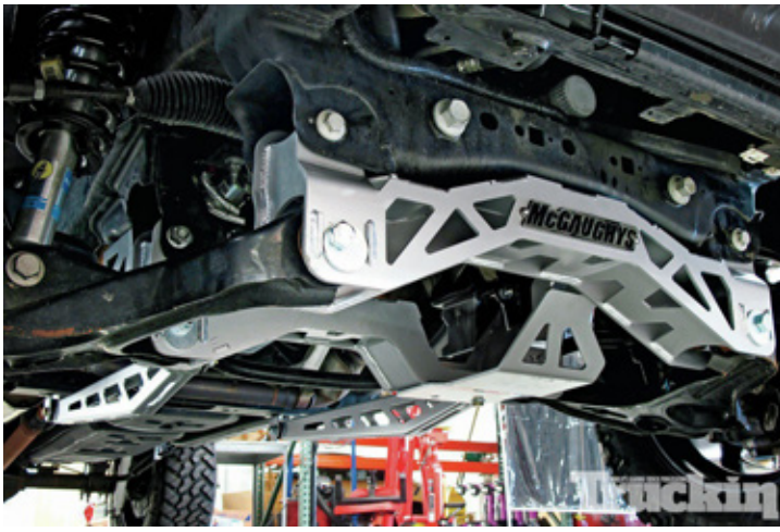
23. All tightened up, we noted how nicely McGaughys had tucked everything to maximize allowable ground clearance.
