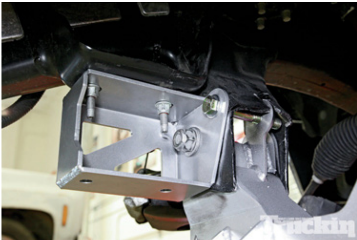
13. McGaughys created these mounts to allow the sway bar to work as designed with its lift system.
