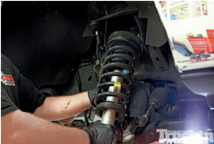
6. We then slipped the struts out of the truck and set them off to the side.
