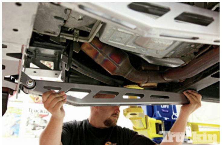
22. Everything was left loose to make installing the compression struts manageable.
