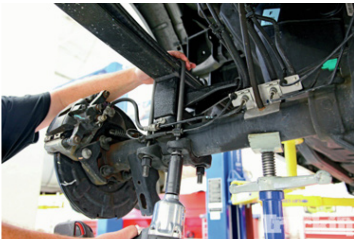
25. With the rear axle supported, the original U-bolts were tossed and the new McGaughys 4 1/2-inch lift blocks were installed with longer U-bolts.
