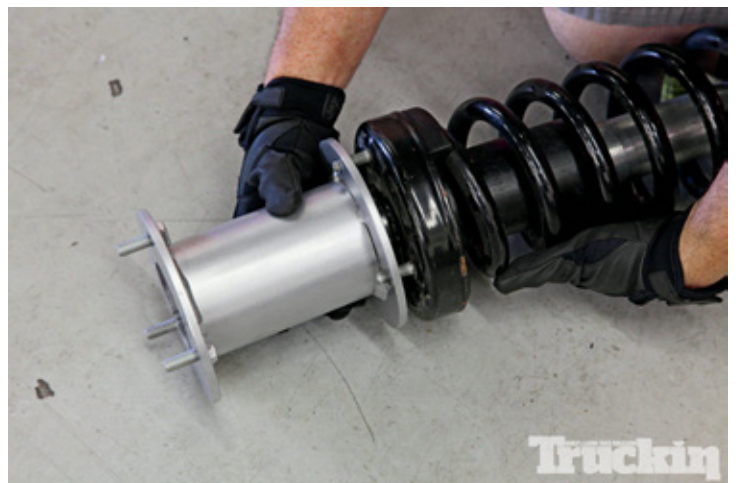
16. Fabricated tubular mounts were added to the struts' upper mounting plate.
