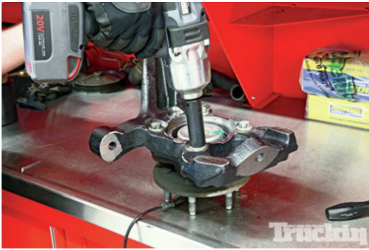
17. Pre-prep work on the workbench had our unit bearings swapped from the old knuckles to the taller McGaughys counterparts.
