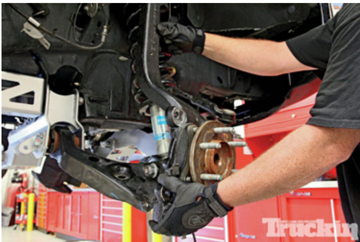
19. The new knuckles dropped right into place between the control arms using the factory ball joint nuts.
