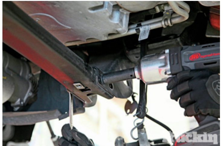
9. One modification needed to be addressed prior to installing any of the suspension lift components. It started with pulling this support crossmember from the Ford.
