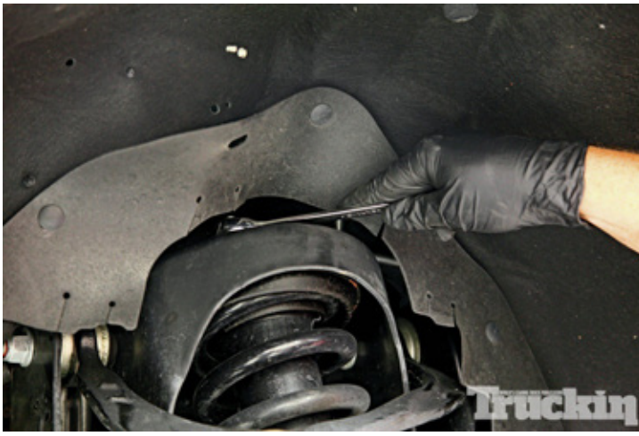
5. The upper and lower hardware holding the Bilstein struts in place was removed.
