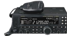
FT-450D A100W HF + 6M Transceiver
