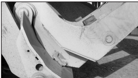
Side View of Subframes and Hooks
