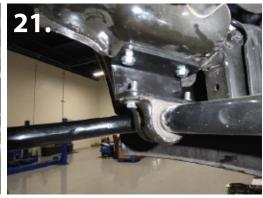
**15.** Install new front sway bar drop brackets using the provided 3/8" x 1" bolts. Install the factory sway bar mounts onto the new drop brackets using the factory hardware. (pic 20-21)
