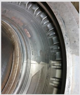
In situ on site cleaning without having to remove the molds. Cleaning when hot is an advantage to the cleaning with dry ice. Quick return of equipment back into production. No need to cool down and reheat.
