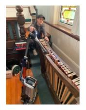
slightly tap a metal slider on a pipe. The ones with scrolls aren't tapped- we just slightly roll or unroll them. This process for each pipe adjusts the pitch of the pipe - aka tuning it!"
